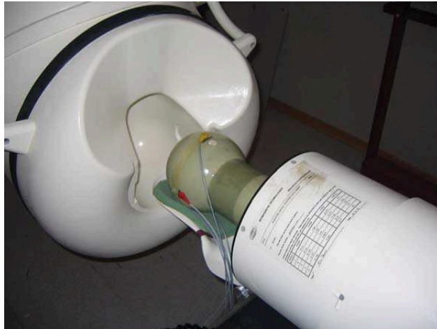
Figure 5.4: The phantom before the measurement in the MEG system. Reference coils are fixed to the head of the phantom in order to measure the positions of the MEG sensors relative to the head.
